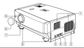
6 Adjustable feet (for adjusting the height and
